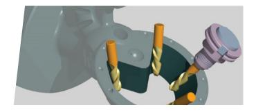
**Tilt to Avoid:** Available in Mastercam's 3D HST Finishing paths, Tilt to Avoid is the fastest way to add Multiaxis motion to a 3-axis toolpath. With just one click, the tool assembly is checked against the machining and avoidance geometries and introduces tilt where necessary to machine the path.
